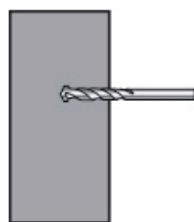
**Please note:** If you are drilling into a tile, it is recommended to tape the wall in the area to be drilled in order to prevent slipping
