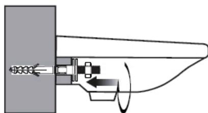
6. Check that the basin is stable then seal along the back edge.
